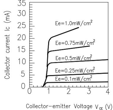
**Typical Electrical/Optical/Characteristics Curves For ITR**
