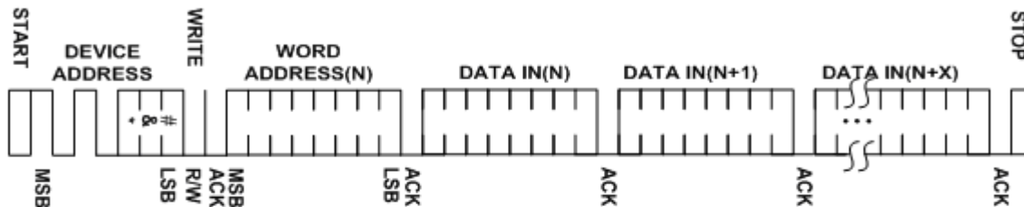
Figure 4: PAGE WRITE INSTURCTION (SDA INPUT)
