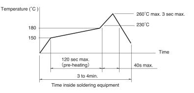
TACT Switch™ Soldering Conditions
