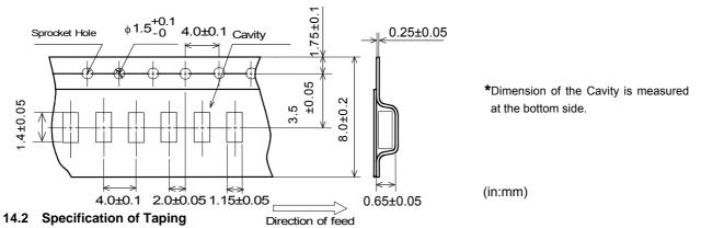
(1)Packing quantity(Standard quantity) 4000 pcs. / reel Direction of feed
