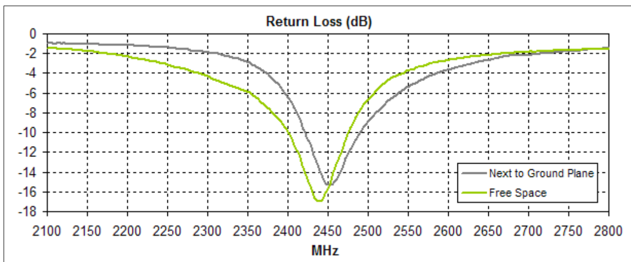
Figure 3. Return Loss for the FXP72 Antenna.
