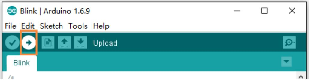
When it is finished the information **Done Uploading** will Pop up in the lower left corner of Arduino IDE.
