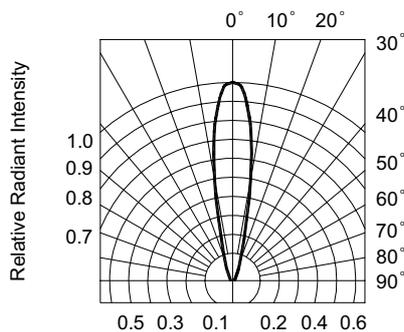
FIG.6 RADIATION DIAGRAM
