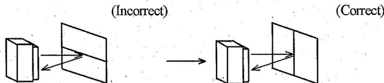
7-7 In order to decrease measuring error due to moving direction of object, we recommend that the sensor be mounted like the drawing below.
