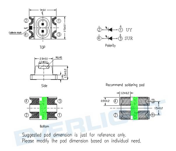
Note: Tolerances unless mentioned ±0.1mm. Unit = mm
