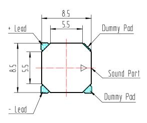
\*Unit: mm; Tolerance: ±0.3mm Except Specified
