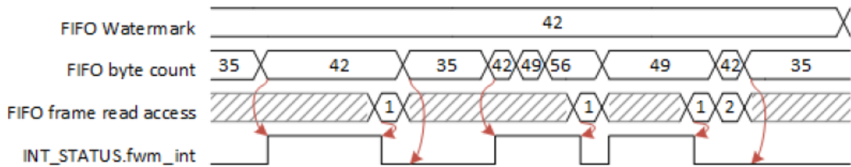
Figure 7: FIFO watermark interrupt, non-latched with reads from FIFO
